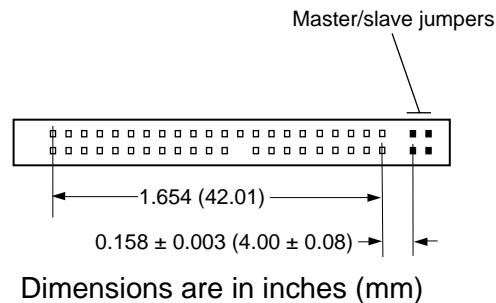
Figure 5. ATA interface connector dimensions (non-SFF dimension, for reference only)
